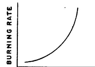
PRESSURE INTRODUCED BY CONFINEMENT OF THE BURNING POWDER
